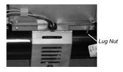
**15)** Before re-attaching the rear access panel, the valve wires and the fan wires need to be connected.
